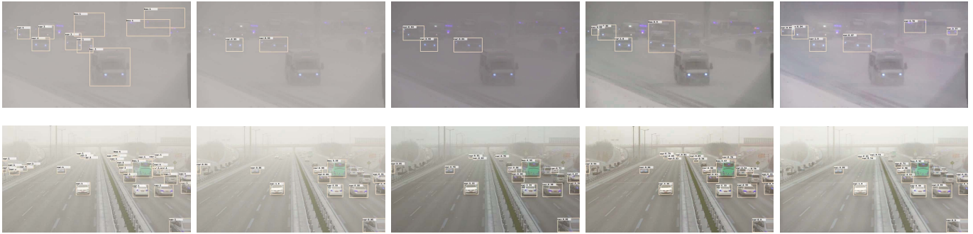
Fig. 7. Examples of object detection of hazy images and dehazed images on RESIDE RTTS set. The first column displays the ground truth bounding boxes on hazy images, the second column displays detected bounding box on hazy image using pretrained Mask R-CNN, the right three columns display Mask R-CNN detected bounding boxed on dehazed images using AOD-Net, MSCNN, DCPDN correspondingly.
